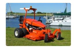
One of the added benefits to the new Kut Kwick Tier 4 machines is the digital information flat screen that provides the operator with all the pertinent engine information. This feature is part of an engine management system that monitors operating parameters and allows the maintenance team to set service interval reminders. As always, Kut Kwick machines have a certified Rollover Protection System (ROPS) for safety and are all true zero-turn-radius (ZTR) machines for maximized productivity.
