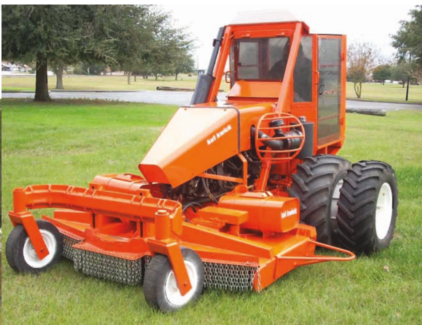
MSM83-88D shown with optional dual rear wheels allow for operation on 40° slopes.
