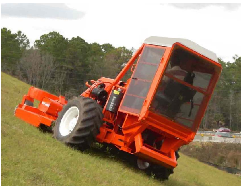
Optional enclosed cab includes A/C (Heat optional).
