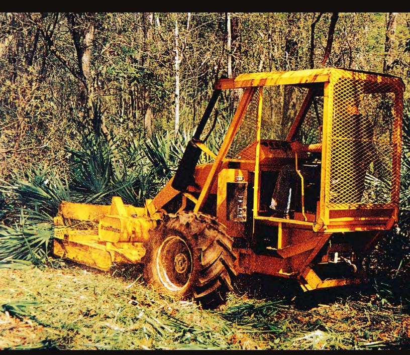
The Kut Kwick BrushMaster (BM) series mower is designed for land developers for the preparation of land for sale and for foresters in the management of woodlands, fire mitigation and fighting, and tree farms. The BrushMaster is capable of removing and mulching brush and trees to 4" in diameter.
